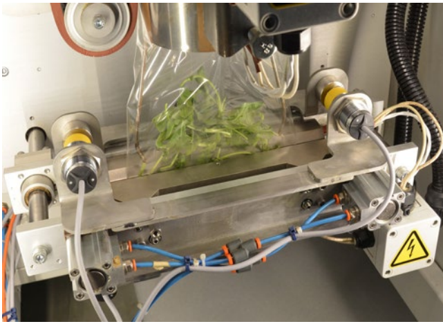
Sensors on the sealing bars measure anomalies such as product in seal, wrinkles, folds that can cause leaks
