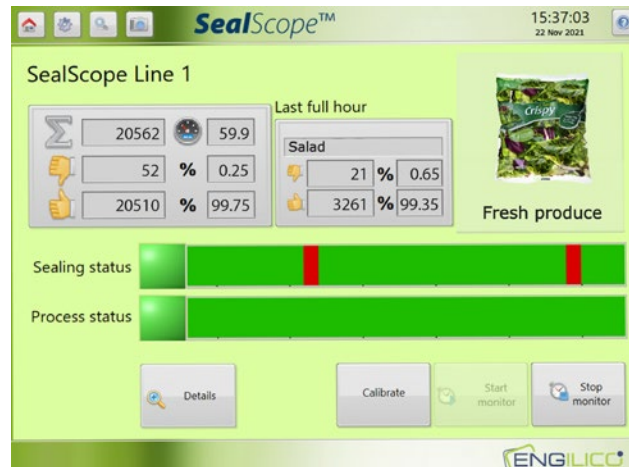
The SealScope™ UI provides basic information on both the individual seal quality as well as the sealing process status
