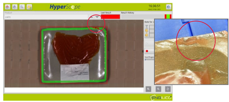
Hyperspectral imaging detects foreign material (e.g. fish, oil) with high contrast in the sealing area of a package with a cardboard backing.
