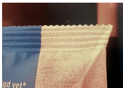
Wrinkles or folds in the seal can lead to leaks in the cheese package
