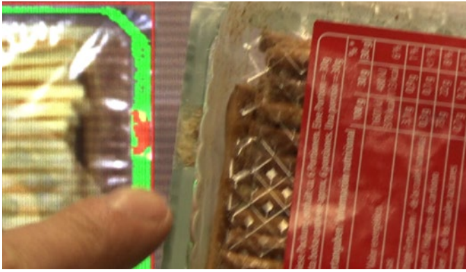
A hyperspectral camera distinguishes materials that have different spectral images, allowing it to recognize contaminations in the seal through printed film.
