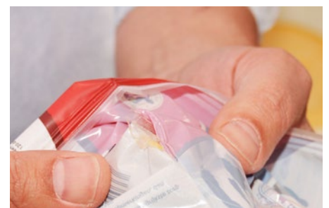
Cheese parts in the seal are retrieved in a package that is rejected by SealScope®
