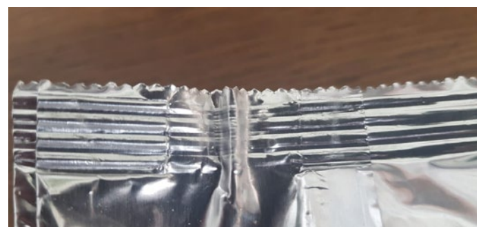
Plies/Fold in seal possibly causing leaking packages
