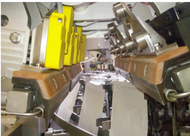
Distance sensors on the sealing bars detect whether there is product or folds in the seal
