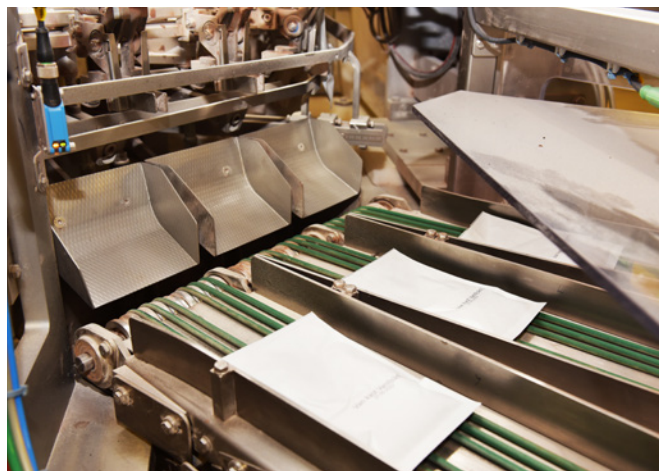
Defective packages are dropped from the belt with a sliding hatch system.
