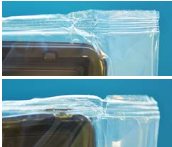
Defective packages rejected by the SealScope™ system with folds (top) and plastic tray in seal (bottom).
