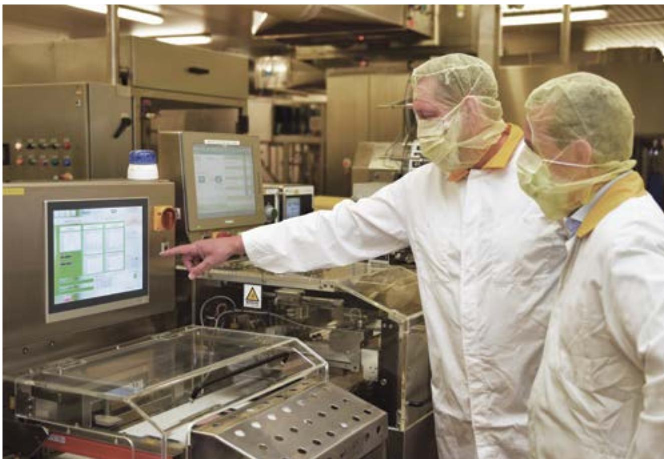
The SealScope™ system provides 100% seal inspection and reveals trends in the packaging process
