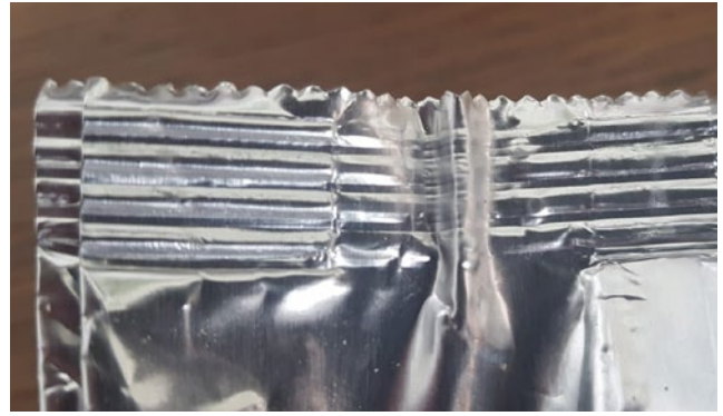
Package with undesired plies rejected by the SealScope ® system
