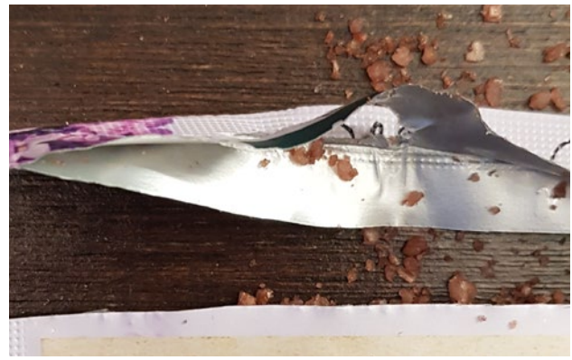
Defective sachet with salt crystals in the seal
