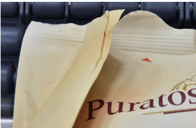
Rejected package due to fold in the seal.
