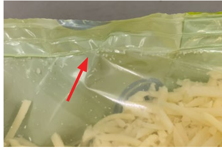
Wrinkles in the seal can lead to leaks in the cheese package
