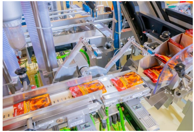
Leaking packages need to be avoided to prevent outgoing product quality issues and the soiling of packaging machinery.
