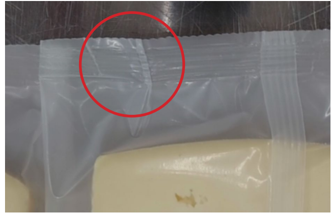
As the cheese wedges are thicker at the end of the package, folds might occur in the seal.
