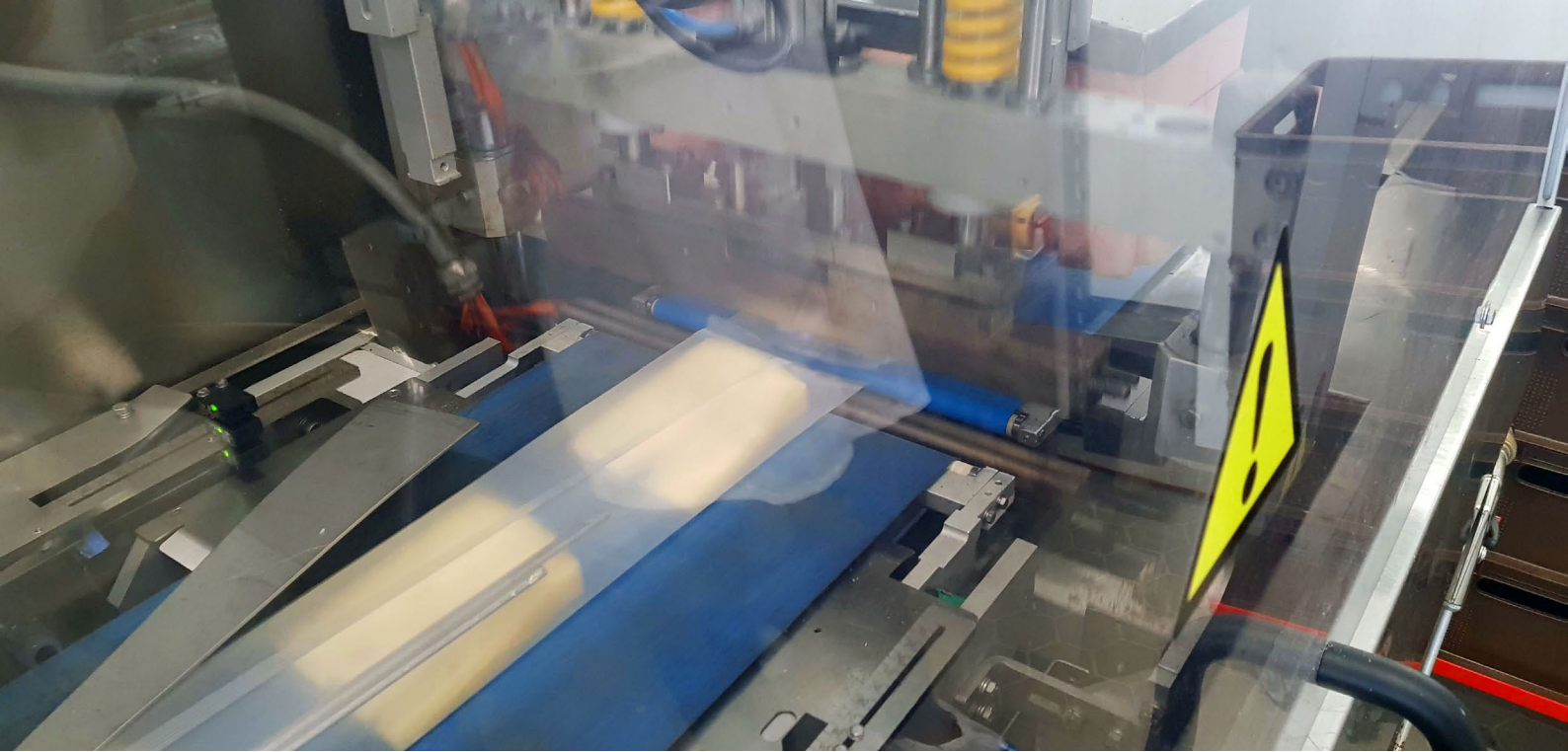
Cheese wedges are MAP packaged on the ULMA FM305 flow-packer.
