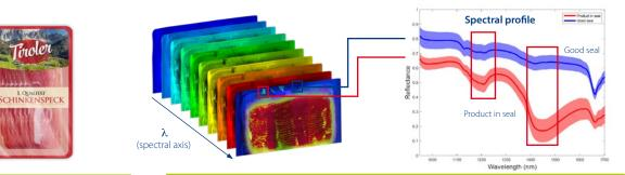
A standard industrial camera image is built from 3 wavelengths ranges (RGB) and only provides visible information The hyperspectral 3D spectral image map is built from a broad wavelength spectrum. Every pixel is analyzed individually and differences in materials or composition are detected, even through printed foil. A contaminated seal has a different spectral profile than the profile of a clean seal.
