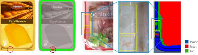
Visual image When product and film have similar colors (yellow-on-yellow), contamination in the seal is hardly visible. Hyperspectral image The higher contrast clearly reveals contamination (red)
