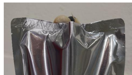
Rejected pouch, due to product in seal
