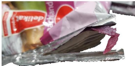
Checking every pouch by hand is a challenge since the production speeds are high and manual labor is costly. This is where SealScope comes in. SealScope is the first in-line, non-destructive, seal inspection device that checks 100% of all top seals. Wrinkles and product are easily detected and can be rejected via a rejection unit. In addition, SealScope continuously monitors the sealing process, providing early warning in case of process drift.
