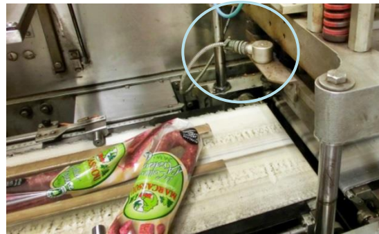
Vibration sensor on sealing jaws
