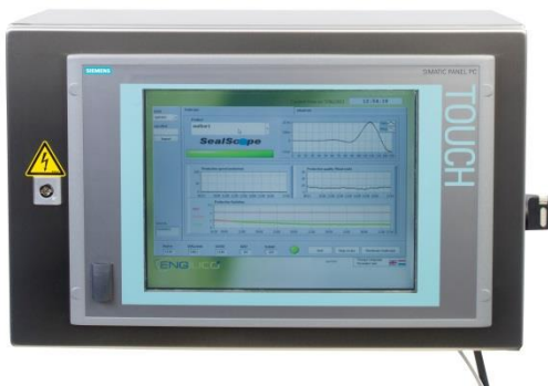
SealScope™ acquisition unit & operator screen
