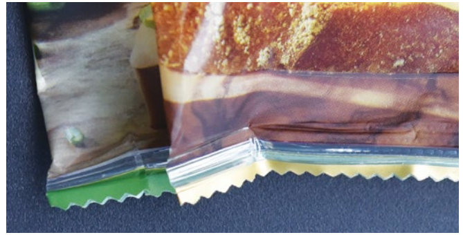
Rejected package with folds in the seal.
