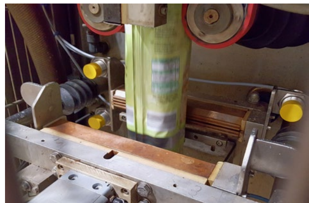
Sensors on the sealing bars
