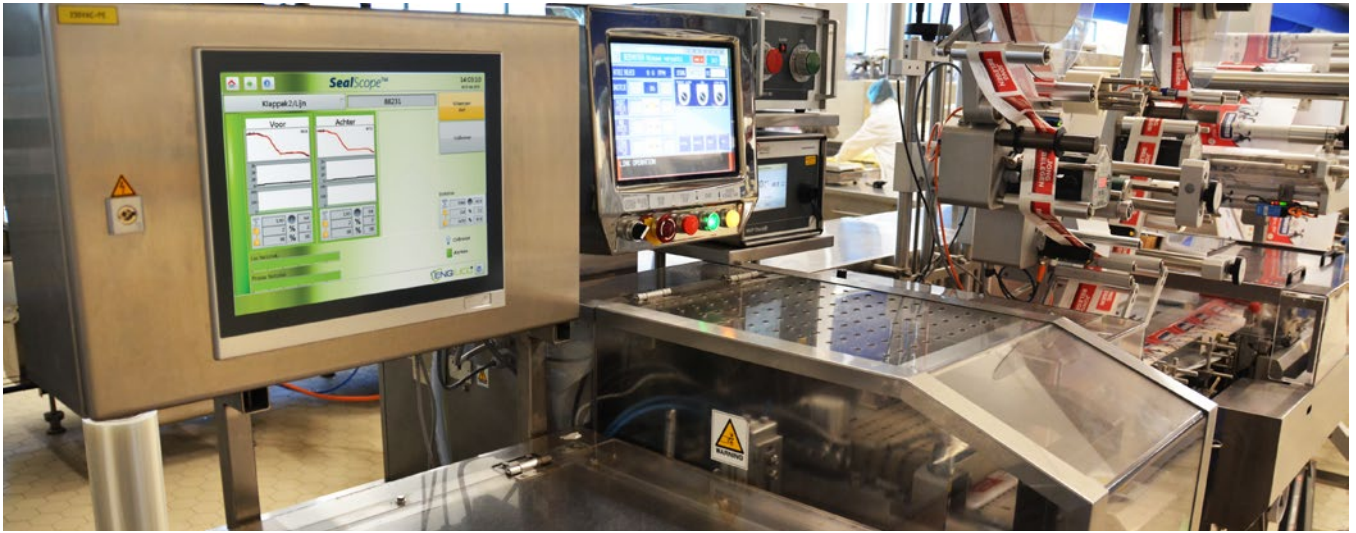
SealScope ® monitoring console in the packaging line
