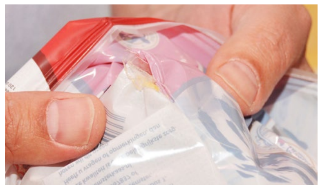
Cheese parts in the seal are retrieved in a package that is rejected by SealScope ®
