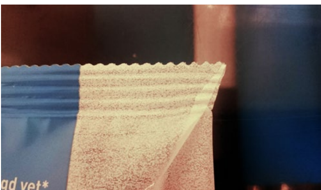
Wrinkles in the seal can lead to leaks in the cheese package
