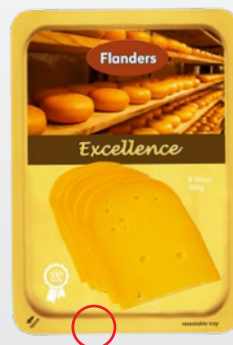
Visual image When product and film have similar colors (yellow-on-yellow), contamination in the seal is not visible
