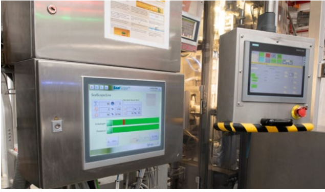
The SealScope ® system is fully integrated into the UVA VFFS machine and requires no additional space in the packaging line.
