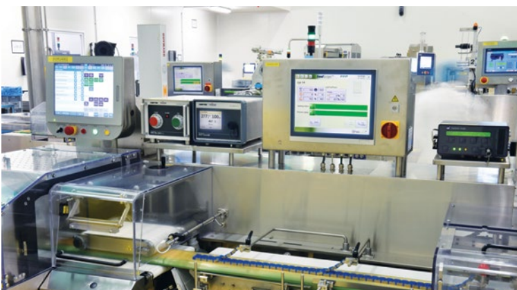
Also the new OMORI flow-pack line is equipped with the SealScope ® seal inspection system.
