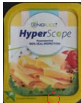
Visual image When product and film have similar colors (yellow-on-yellow), contamination in the seal is not visible
