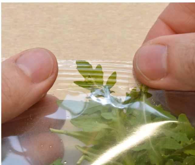
Product in seal causing leaking packages
