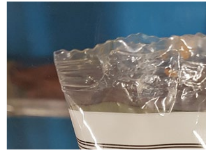
Handl Tyrol uses SealScope™ to inspect flow-packs with sausages (left); Folds ((middle) or product (right) in the sealing area can lead to leaking packages
