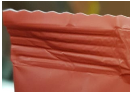
Handl Tyrol uses SealScope™ to inspect flow-packs with sausages (left); Folds ((middle) or product (right) in the sealing area can lead to leaking packages
