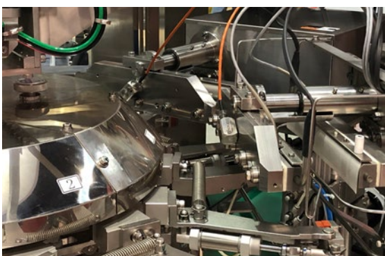
SealScope™ sensors on the sealing bars of a rotating pouch machine
